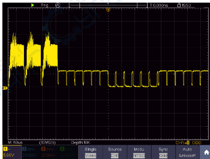
Figure 8-7 Waveform Captured from Video Field Trigger
